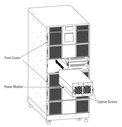
Figure 73. Power Module Replacement
