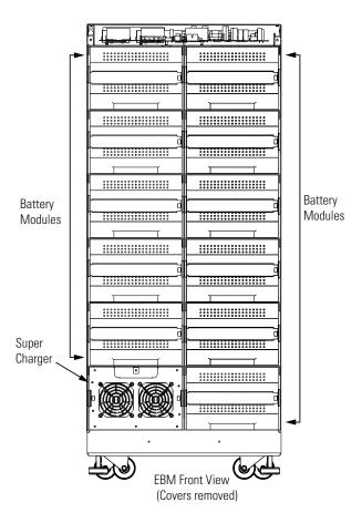
Figure 47. EBM Battery Modules and Charger
