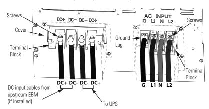
Figure 37. Battery Cable Assembly Installation.
