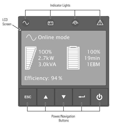
Figure 6. UPS Control Panel
