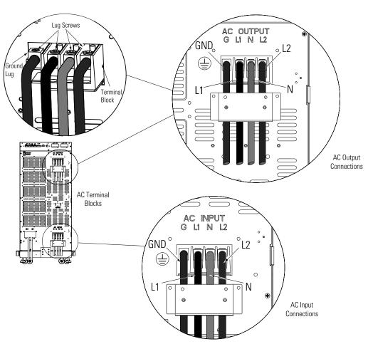
Figure 34. UPS Input and Output Terminal Connections
