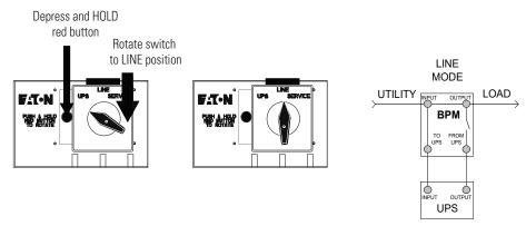
Figure 26. Bypass From UPS to LINE
