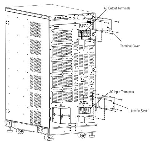
Figure 15. UPS AC Power Terminal Access
