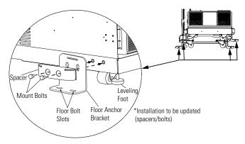
Figure 9. Floor Anchor Bracket Installation
