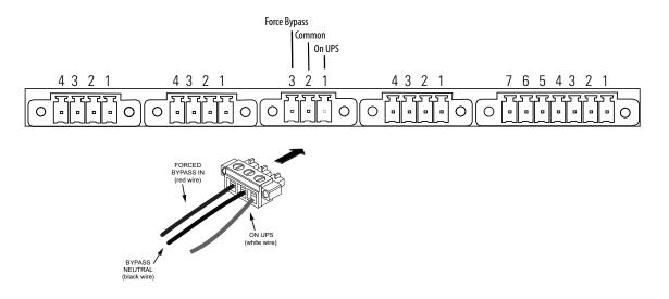
Figure 21. Three-Pin BPM to UPS Connector
