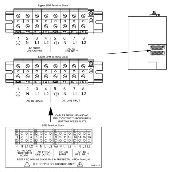
Figure 18. Bypass Switch Wiring Label and Terminal Blocks
