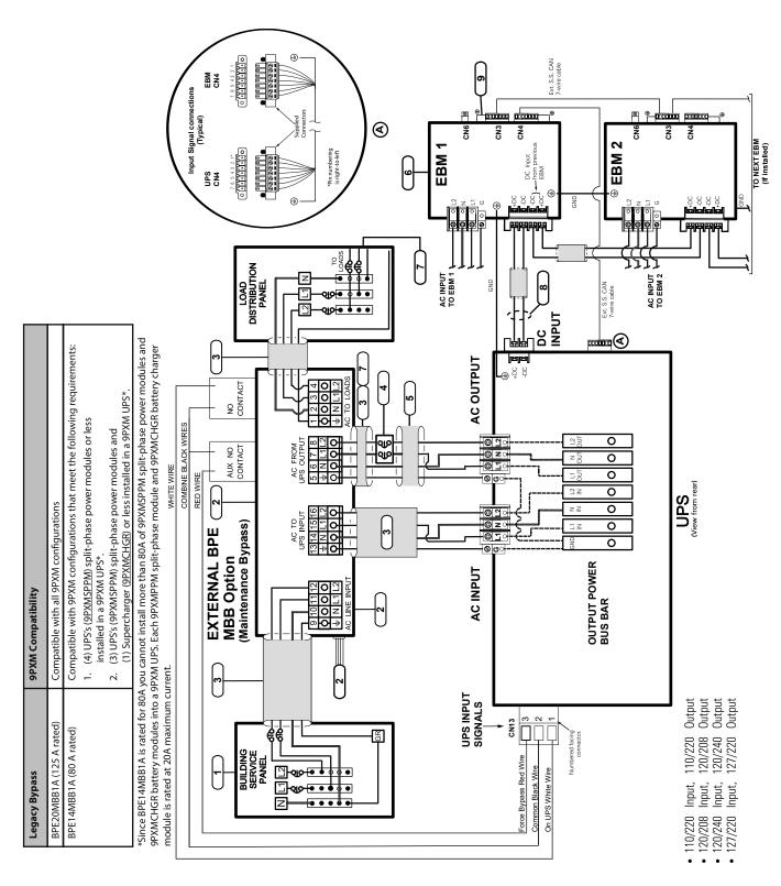
Figure 24. Wiring Diagram - UPS with External Bypass Switch (L1, L2, N) and MBB Option
