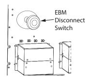
Figure 45. EBM Emergency Disconnect Switch
