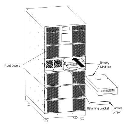
Figure 72. Battery Replacement
