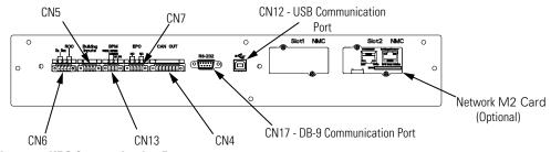
Figure 68. UPS Communication Ports
