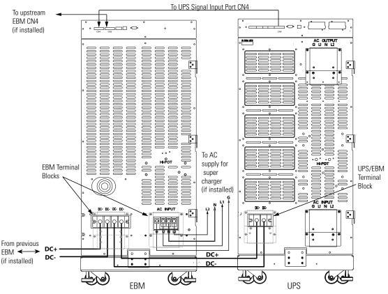
Figure 41. EBM to UPS Connections
