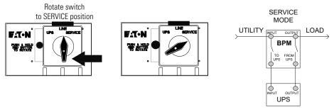
Figure 27. Bypass From LINE to SERVICE
