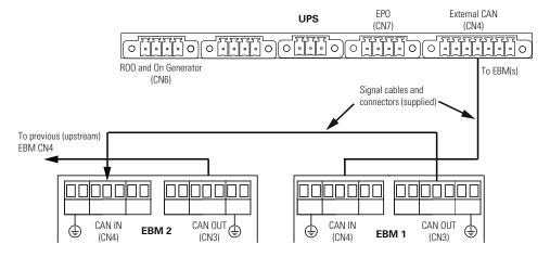
Figure 42. UPS Input Control Signal Wiring (for External Controls)
