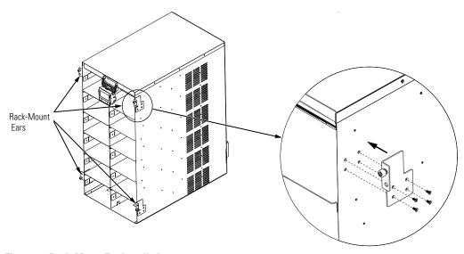
Figure 10. Rack-Mount Ear Installed
