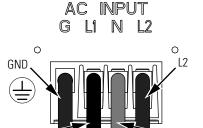
Figure 33. UPS Input Wiring
