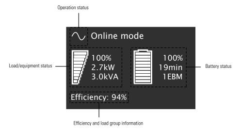
Figure 50. LCD Display Status Indicators
