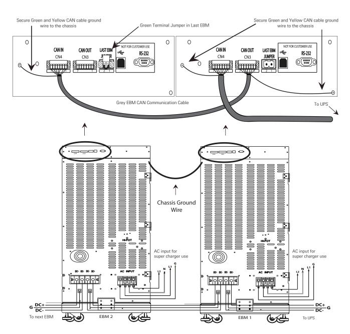
Figure 44. CAN Communication Wires UPS to EBM
