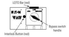
Figure 25. Bypass Switch Positions
