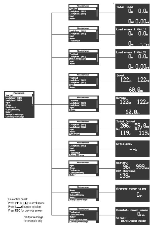
Figure 55. Measurements Menu
