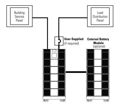
Figure 31. Typical Installation without a Bypass Switch
