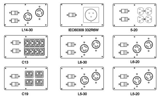
Figure 74. Compatible Output Receptacles
