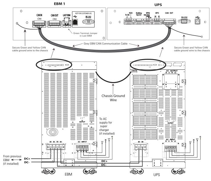
12. Close the DC emergency disconnect switch button on the back of each EBM. Insert the switch key supplied with the cabinet into the button and turn clockwise 1/2-turn. Pull the button OUT to close the switch and reconnect DC power. Turn the key back counter-clockwise, and remove the key (see Figure 44)
