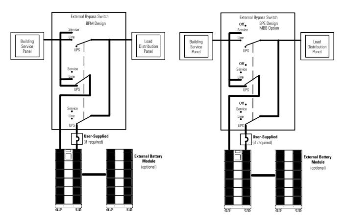
Figure 14. Typical Installation with a Bypass Switch
