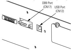
**Figure 48. Communication Ports**
