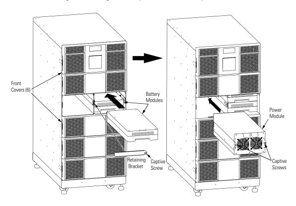
Figure 46. Inserting the Modules
