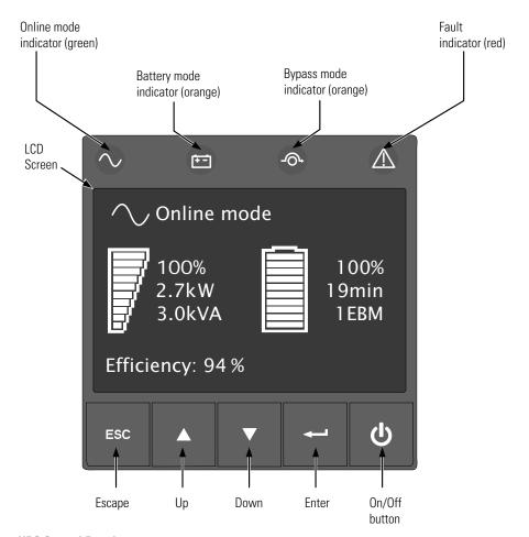
Figure 49. UPS Control Panel
