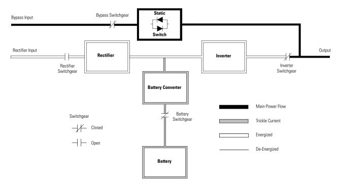
Figure 5-2. Path of Current Through the UPS in Energy Saver System Mode
