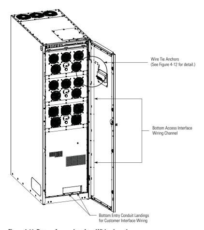
Figure 4-11. Bottom Access Interface Wiring Location
