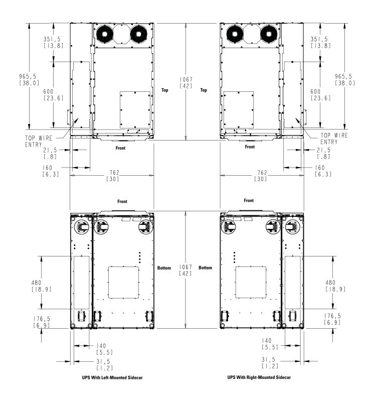
Figure 3-5. UPS Cabinet with Left-Mounted or Right-Mounted Sidecar Dimensions (Top and Bottom Views)
