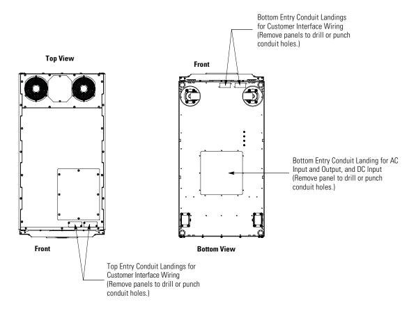
Figure 4-4. UPS Conduit and Wire Entry Locations
