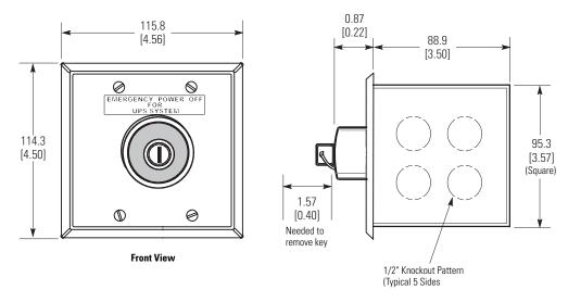
Figure 3-8. Remote EPO Switch Dimensions
