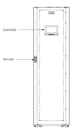
Figure 6-1. UPS Controls and Indicators
