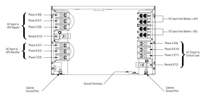
Figure 4-8. Power Terminal Detail
