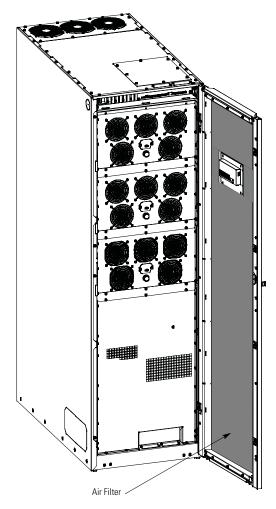
Figure 8-1. Air Filter Location
