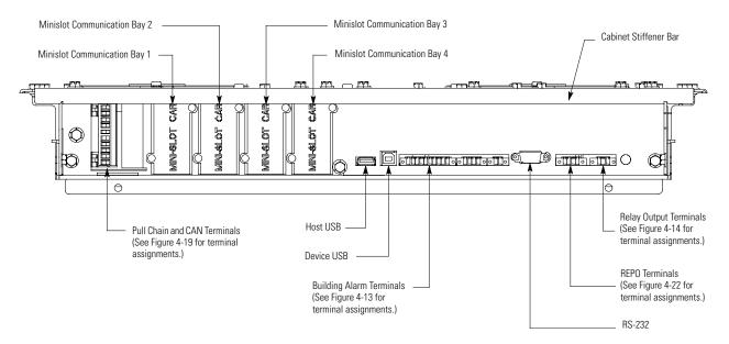
Figure 4-10. Interface Terminal Detail
