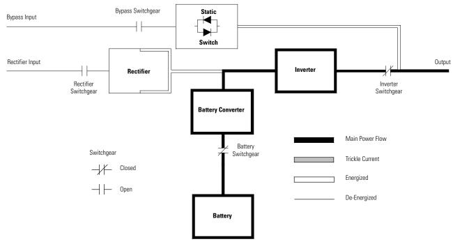
Figure 5-5. Path of Current Through the UPS in Battery Mode
