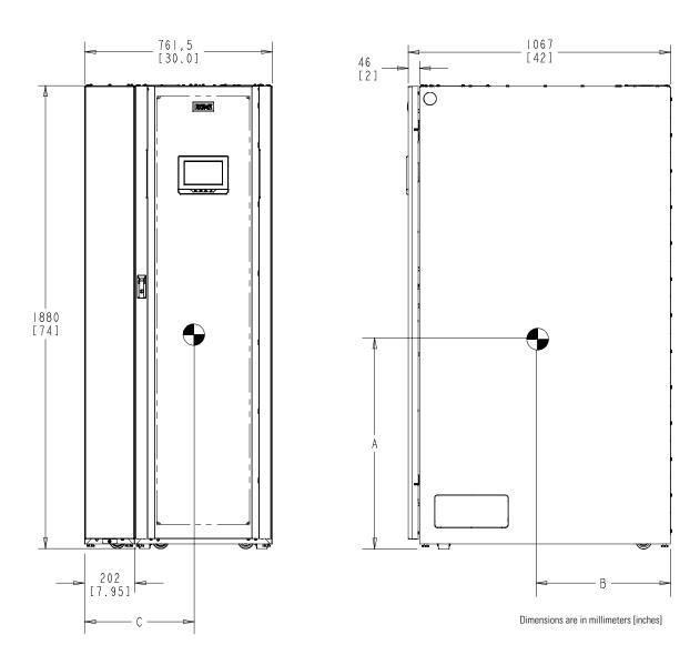
Figure 3-7. UPS Cabinet with Left-Mounted or Right-Mounted Top Entry Wiring Sidecar Center of Gravity
