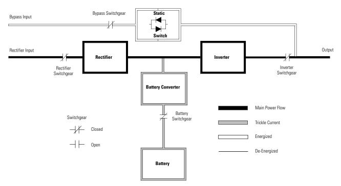
Figure 5-3. Path of Current Through the UPS in Normal Mode
