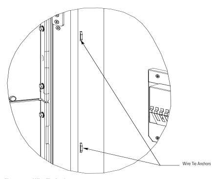
Figure 4-12. Wire Tie Anchors
