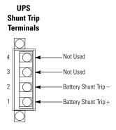
Figure 4-17. Battery Shunt Trip Terminal Assignments
