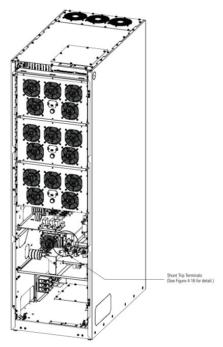
Figure 4-15. Battery Shunt Trip Locations
