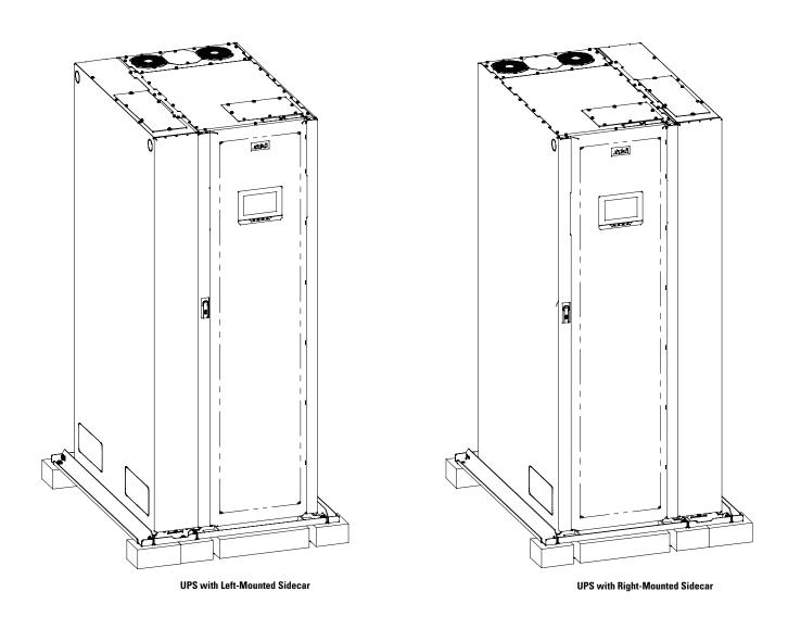
Figure 3-11. UPS Cabinet with Left-Mounted or Right-Mounted Top Entry Wiring Sidecar as Shipped on Pallet
