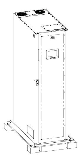
Figure 3-10. UPS Cabinet as Shipped on Pallet
