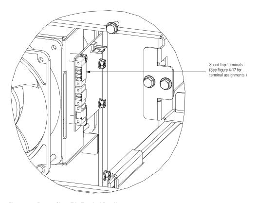
Figure 4-16. Battery Shunt Trip Terminal Detail
