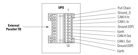
Figure 4-19. External Parallel Terminal Block
