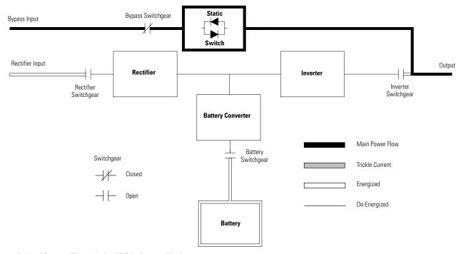
Figure 5-4. Path of Current Through the UPS in Bypass Mode
