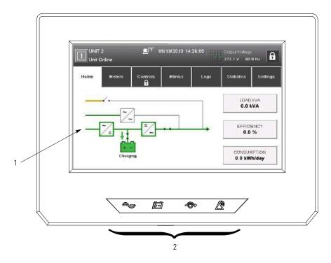
Figure 6-2. UPS Control Panel
