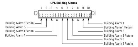
Figure 4-13. Building Alarm Terminal Block Connector Assignments
